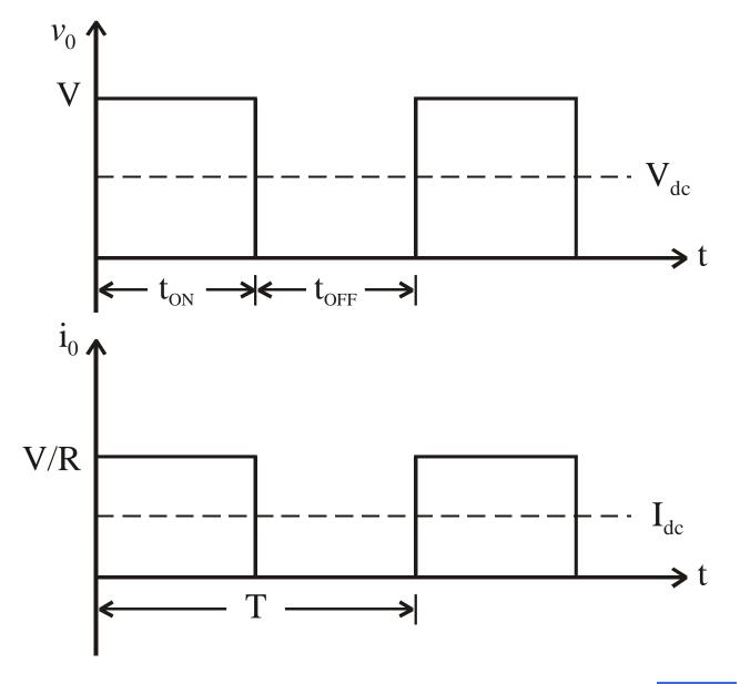
$V_{dc}$  = Average value of output or load voltage.
