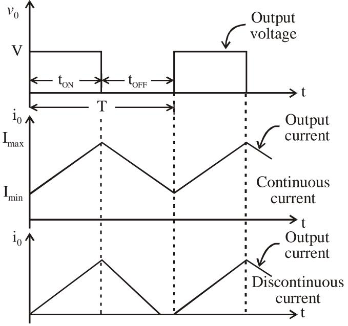
Expressions For Load Current  $i_O$  For Continuous Current Operation When Chopper Is ON  $(0 \le t \le t_{ON})$
